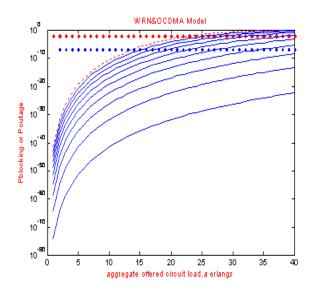
Fig. 6. Plot for  $P_{outage}$  or  $P_{block}$  Vs aggregate offered circuit load with K = 64 subscribers,  $\Gamma$ = 32 channels  $p_{outage}^{max} = 10^{-6}$  and  $p_{blocking}^{max} = 10^{-2}$ .
