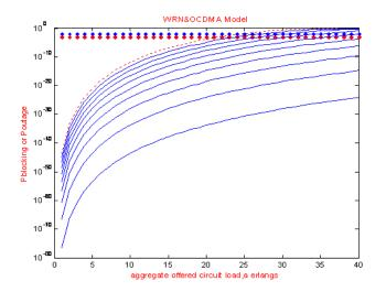
For K= 64 subscribers and  $\Gamma$ = 32 channels, the  $p_{outage}^{max} =$ constraint  $10^{-6}$ operating are and  $p_{blocking}^{max} = 10^{-2}$ , the graph between aggregate carried circuit load and Poutage is given in Fig.6 with circuit activity ranging from 10% to 90% and traffic capacity Vs circuit activity p is given in Fig. 2(b). The  $p_{outage}^{max} =$ operating constraint are  $10^{-6}$ and  $p_{blocking}^{max} = 10^{-2}$ .
