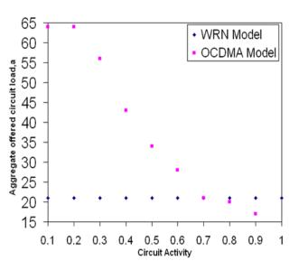
Fig. 7. Aggregate offered circuit load Vs Circuit activity with K = 64 subscribers,  $\Gamma$ = 32 channels  $p_{outage}^{max} = 10^{-6}$  and  $p_{blocking}^{max} = 10^{-2}$
